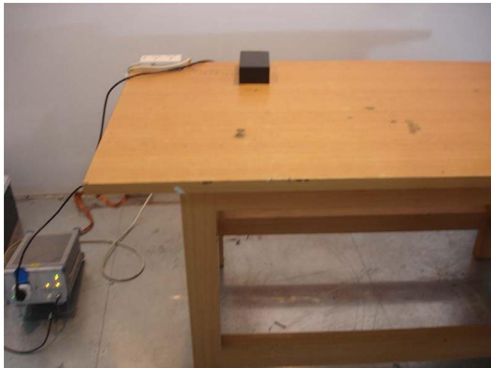
**Photo 2 Radiated Emission Test Setup**
